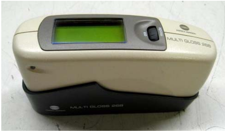
Fig.2.15 Photograph of glossmeter GM-268.
