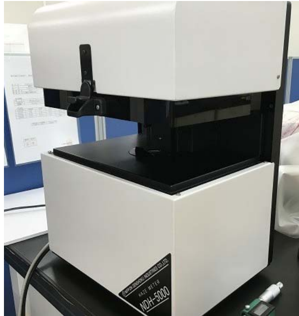
Fig.2.21 Photograph of hazemeter NDH5000.
